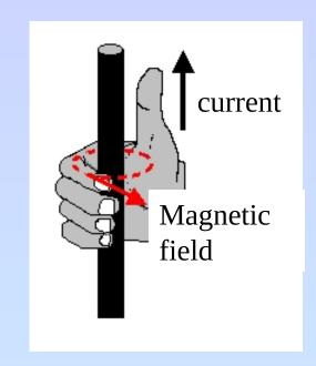
If you reverse the direction of the current, the direction of the magnetic field reverses also
