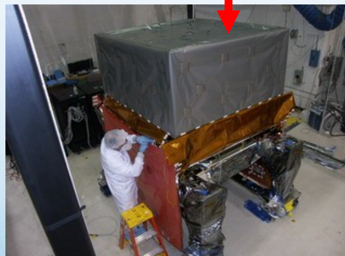
Integrated LAT with radiators
