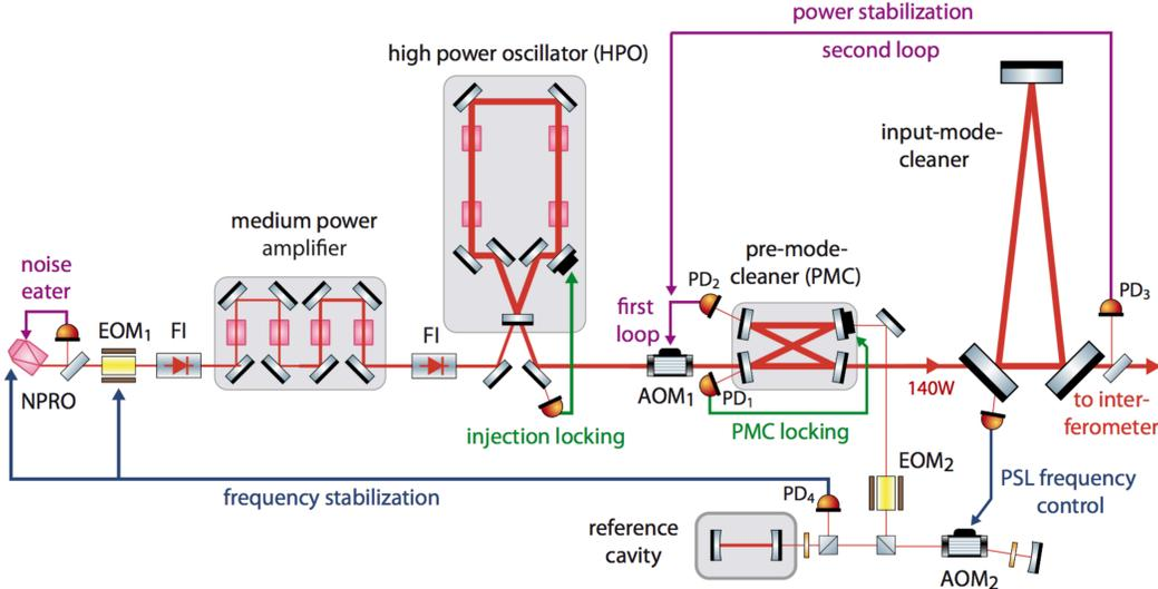
**Figure 4** Schematic of the pre-stabilized laser system. The Input Mode Cleaner is discussed in section 4.2. AOM: acousto-optic modulator; EOM: electro-optic modulator; FI: Faraday isolator; PD: photodetector.
