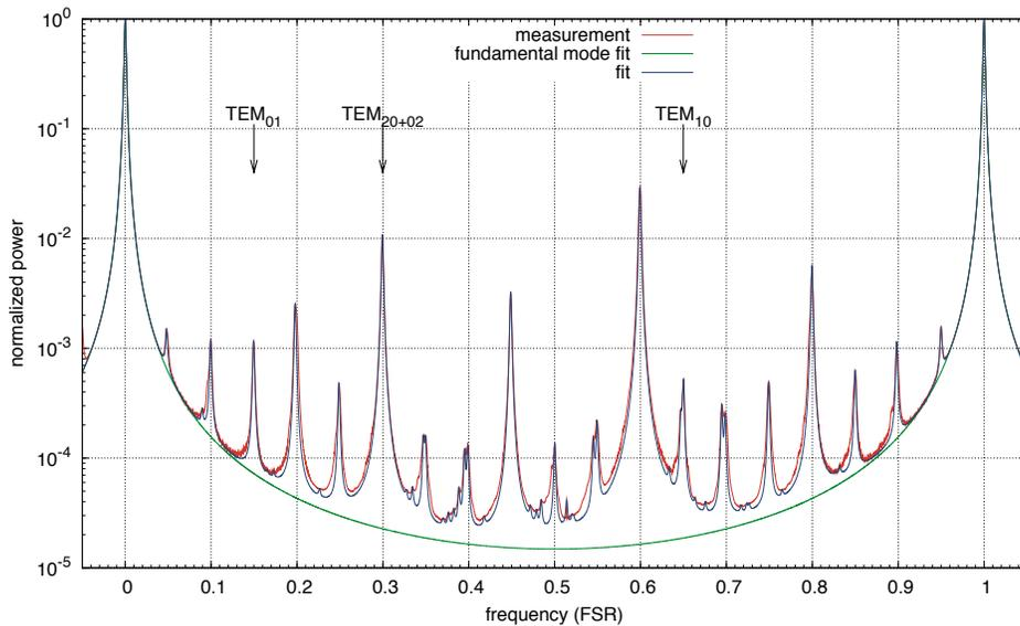
**Figure 5** Mode scan of the high power laser used on the L1 interferometer. Close to 95% of the power is in the TEM<sub>00</sub> mode.
