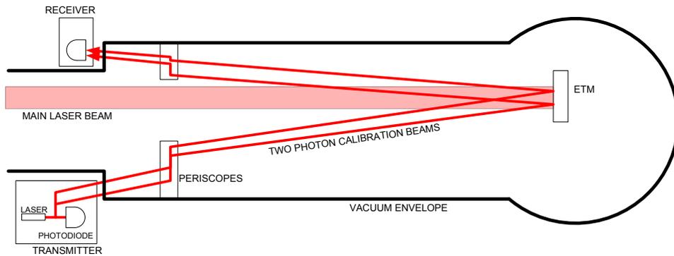
**Figure 19** Schematic of the photon calibration system.
