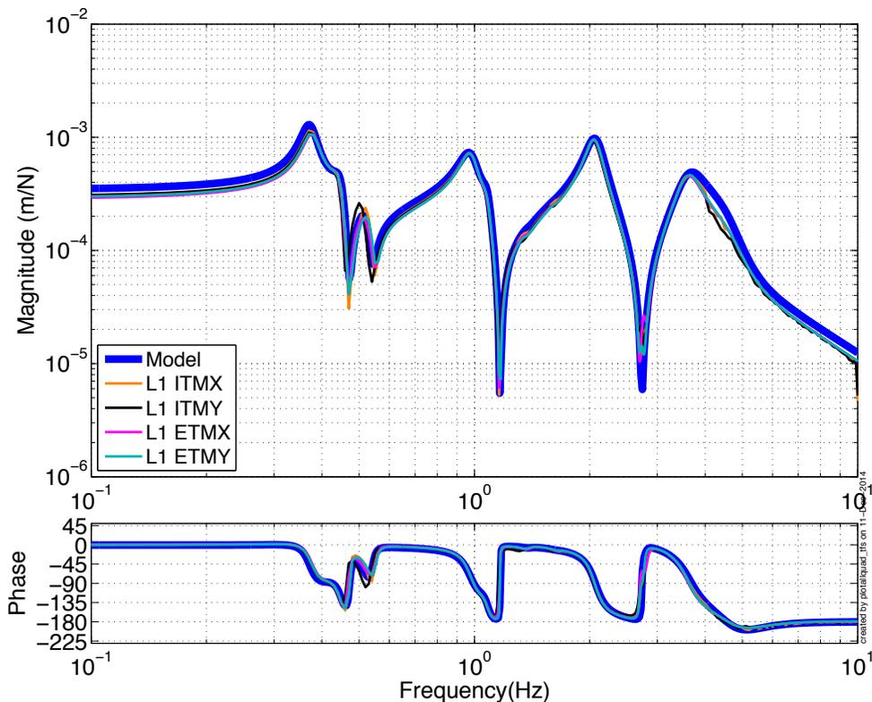
**Figure 9** Transfer functions from longitudinal force to longitudinal position of the top mass for the four test mass suspensions at LLO. Active local damping is engaged for these measurements; the suspension model curve shows good agreement with the data.
