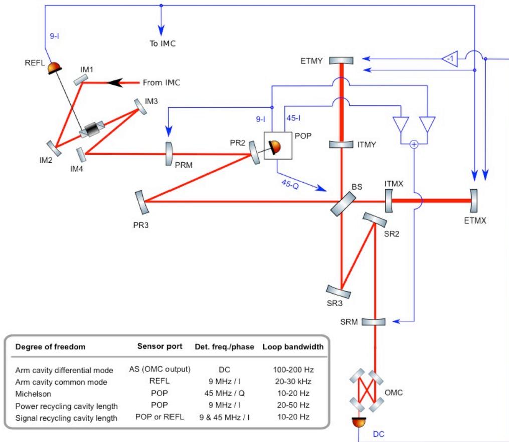
**Figure 15** Length sensing and control scheme for Advanced LIGO. Though not shown, the Michelson signal is also fed back to the PRM and SRM, so that the BS actuation affects only the Michelson degree-of-freedom.
