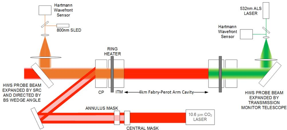
**Figure 13** Schematic layout of the Thermal Compensation System for the X-arm. A similar configuration is implemented on the Y-arm, with the SLED probe beam instead transmitting through the BS. Each of the masks can be independently flipped in or out of the beam path.
