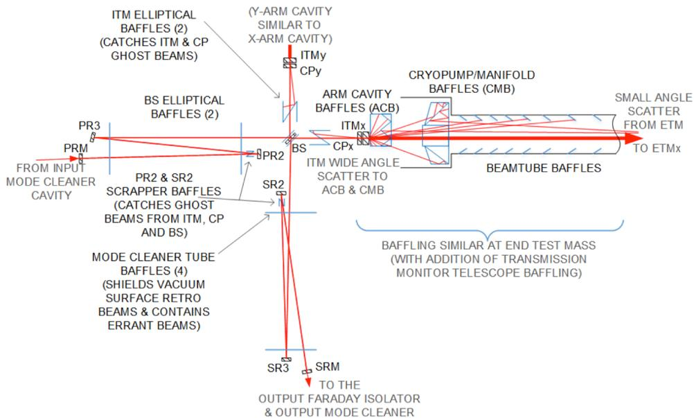
**Figure 14** Locations of the primary scattered light baffles.
