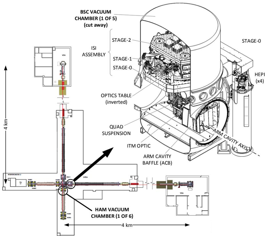
**Figure 10** An Input Test Mass (ITM) vacuum chamber.
