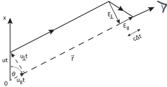
Figure 3: The electric field resolved into components parallel and perpendicular to the radius vector.[1]
