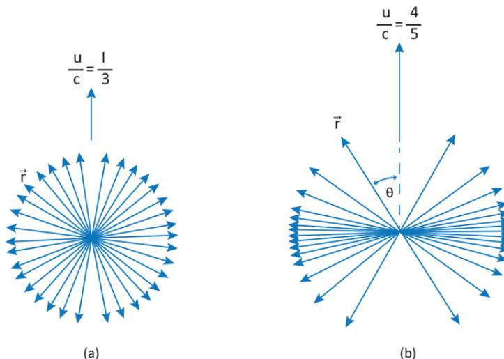
Figure 1: Electric field lines for positively charged particle moving at a constant velocity.[1]
