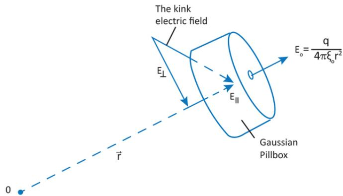
Figure 4: Gaussian pillbox geometry.[1]
