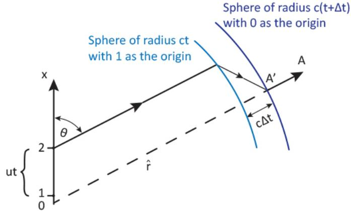
Figure 2: Electric field lines for positively charged particle accelerating for a short time.[1]
