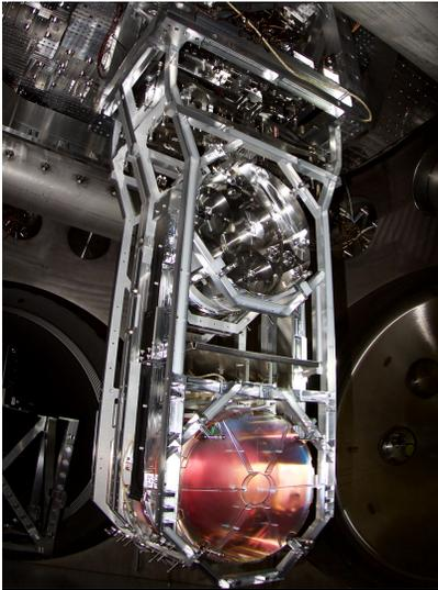
Figure 4.2: The suspension mechanism for the LIGO test masses. At the bottom is one of the test masses (the mirror). Above it can be seen the other elements of the four-stage pendulum that is used to isolate the test mass from ground vibration. Credit: Caltech/MIT/LIGO Lab
