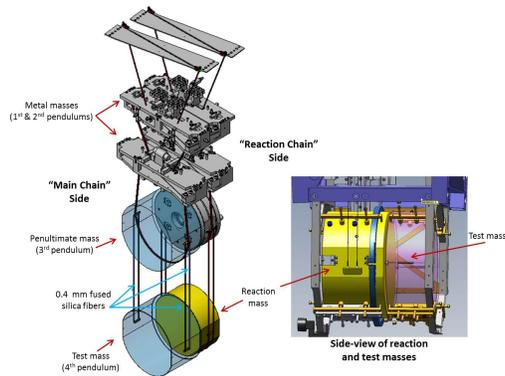
Figure 4.1: The LIGO test masses are suspended in a four-stage pendulum that uses active and passive elements to isolate the masses from ground vibration. The first three pendulums are suspended with metal chains. The last one uses fused silica fibers to help eliminate thermal noise. Image Credit: Caltech/MIT/LIGO Lab
