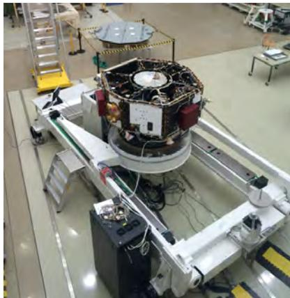
Figure 5: The LISA Pathfinder science module in a clean room in Germany. The large central cylinder is the core assembly for the LISA Technology Package. One of two (gold coloured) colloidal micro-Newton thrusters, provided by NASA, can be seen on the left side of the spacecraft. Credit: ESA – U. Ragnit
